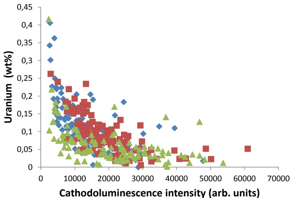
**Fig. 2.** Scatter plot of uranium concentration versus cathodoluminescence intensity, for three different zircon concentrates. Bright zircons (red areas in Fig. 1) typically contain low uranium impurities and hence are likely to have undergone less metamictisation. Low CL intensity (blue areas/grains in Fig. 1) is associated with a high degree of metamictisation.
