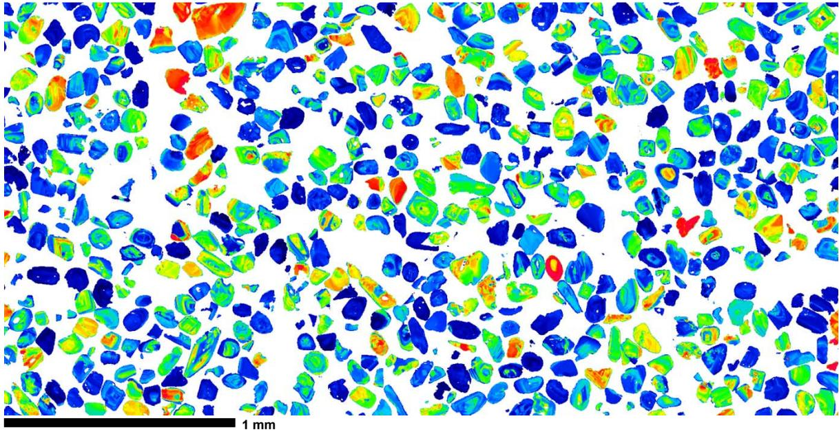
**Fig. 1.** Cathodoluminescence image of zircon grains showing a range of different growth histories and recrystallisation as revealed by CL. The image illustrates the sensitivity of the CL imaging technique to identifying structural and chemical changes within zircon.
